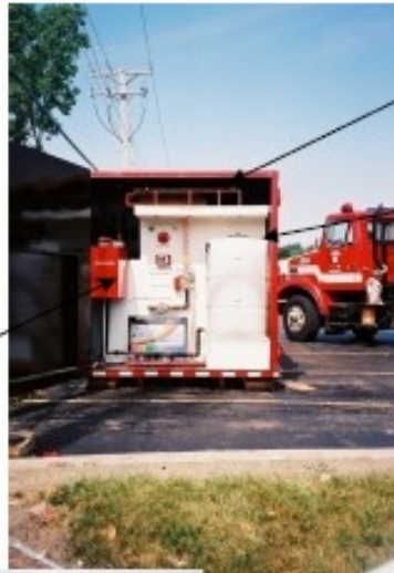
Simulated NFPA 13D Riser
